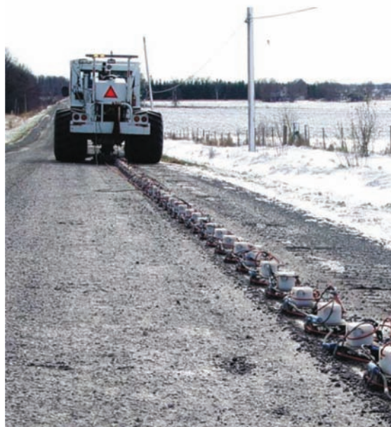
Rys. 7. Pomiary landstreamerem 3C [20]
