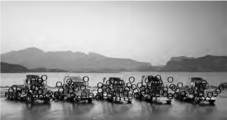
Fig. 3. Keypoints detected by the SURF algorithm. The circles represent the position of the keypoints
