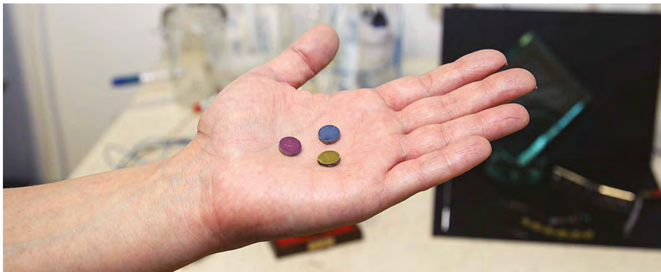
Implant alloy samples of Ti15Mo with hybrid coatings deposited in various electro-chemical conditions / Photo. Małgorzata Kłoskiewicz
