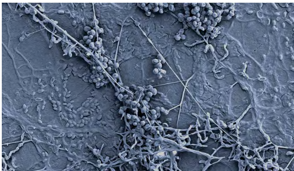
Biodegradation of plastic surface (polyethylene film) by microorganisms (bacteria, fungi, filamentous fungi), magnification 2000× / Photo and coloring: Jagna Karcz
