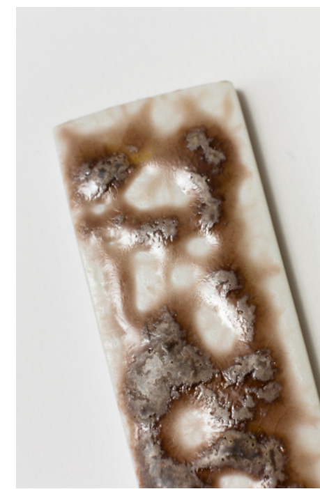
Tests with slag after firing, photo by Barbara Kubska
