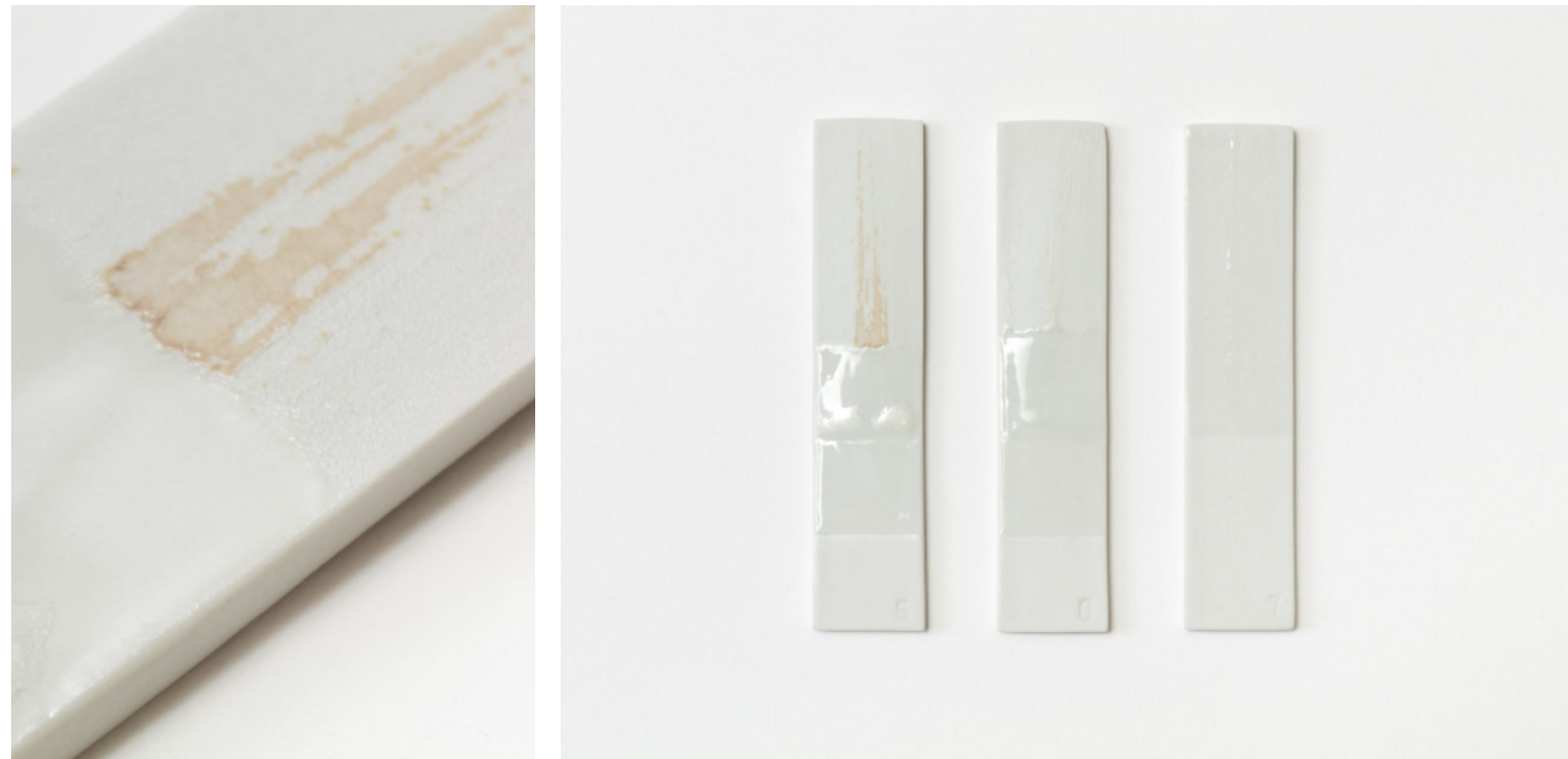
Tests with sand particles after firing, photo by Barbara Kubska
