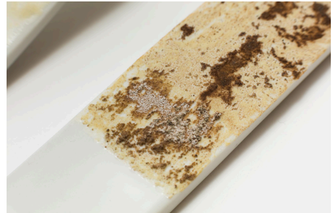
Dolomite tests after firing, photo by Barbara Kubaska
